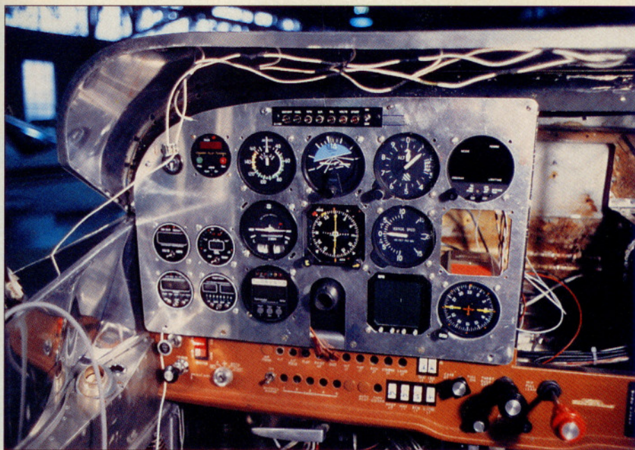
Before painting and placarding, the panel is checked for proper fit. The original subpanel is kept, but the old Cessna rocker switches will be tossed out in favor of new circuit-breaker switches.
