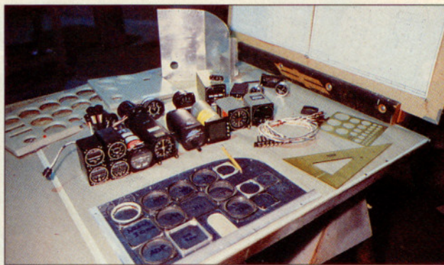
Tracing of the instrument faces on the back of the metal assures an accurately sized hole after cutting.
