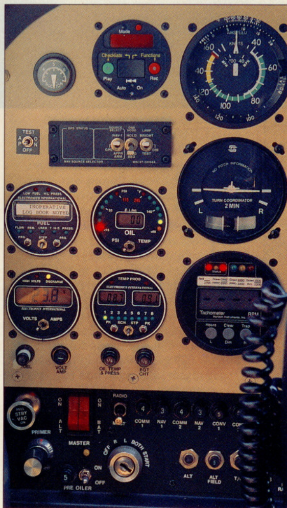
PCR Systems digital voice/clearance recorder and clock, MSI Avionics GPS annunciators, quartet of Electronics International gauges, and Horizon P-1000 electronic tach fit neatly into the left panel.
